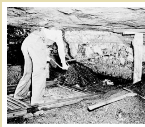
With a hand auger, a miner drills a void for powder charges at the Wheelwright Mine, Floyd County, Kentucky.
